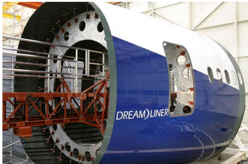
787-8 Fuselage “One Piece” Barrel Test Article
